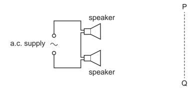
A microphone is moved along the line PQ.
