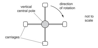
A motor rotates the central pole about its axis. This results in the four carriages each moving along a circular path.
